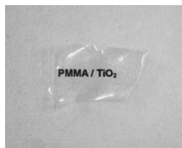
Figure 4. Photograph of 30 wt % \text{TiO}_2 -contained hybrid film.
